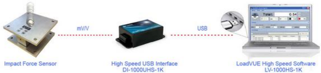
Figure 25. How the impact force measurement system works
