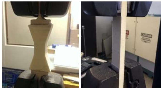
Figure 9. Polyisocyanurate foam characterization – uniaxial tensile test
