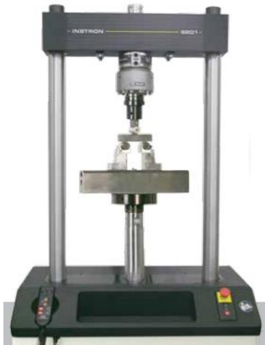
Figure 23. Instron servohydraulic system 8801
