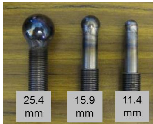
Figure 20. Spherical indenters used in lab measurement
