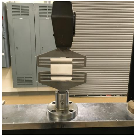
Figure 8. Uniaxial tensile test to TPO membrane with fiber scrim reinforcement
