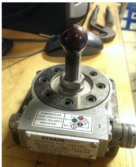
Figure 21. Load cell for quasi-static indentation tests
