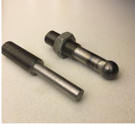
Figure 32. Indenter with flat head D = 9.5\text{mm} (left) with spherical head D = 15.9\text{mm} (right)
