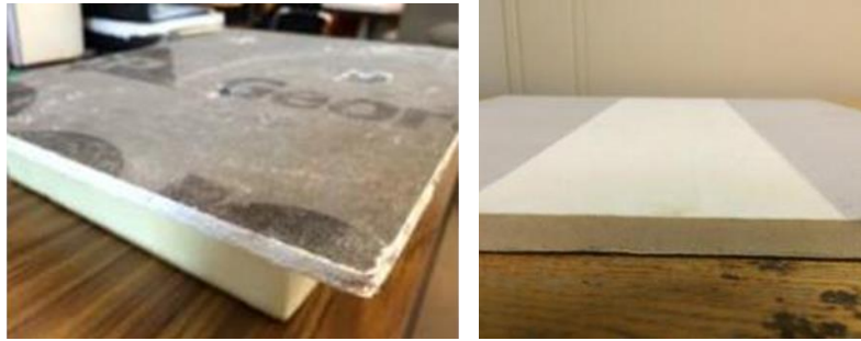
Figure 53. Rigid board: densdeck (left), HDboard (right)
