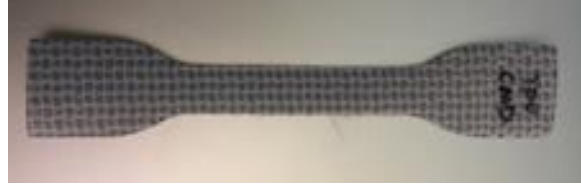
Figure 34. Transparent TPO membrane with fabric scrim reinforcement
